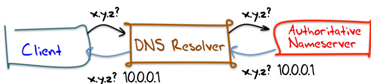
Figure 1 - A Naive view of DNS Resolution
